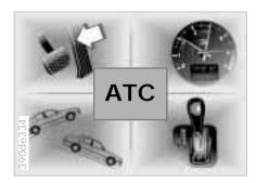
On vehicles with automatic transmission, Adaptive Transmission Control (ATC) uses a number of factors to calculate the gear which provides the maximum efficiency. In this process it monitors your personal driving style, the situation in which you are driving, the condition of the road and the traffic conditions.
