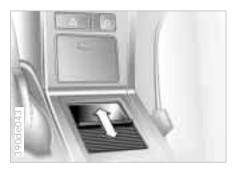
The cover of the storage compartment on the vertical surface of the center console can be pushed open or closed (illustration). If your vehicle is equipped with a cassette holder\*, open each cassette compartment by pressing on the small button.
