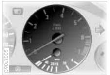
Indicates current fuel consumption in mpg (in liters per 100 km on Canadian vehicles). This instrument shows whether your current driving style is conducive to fuel economy with minimum exhaust emissions.
