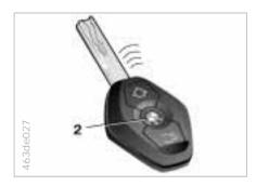
Deactivate the tilt sensor alarm system and interior motion sensor
