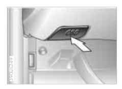
The Onboard Diagnostic (OBD) connector is located on the left of the driver's side at the bottom of the instrument panel and under a cover (arrow).
