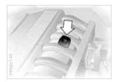
4 Start by connecting the jumper cable from the positive terminal of the support vehicle to the positive terminal connector located in your BMW's engine compartment. The cover of the auxiliary terminal for jump starting is marked with a "+" sign (refer to the illustration). Remove the cover by pulling tab. The illustration shows the external start support point of the BMW 528i. For the BMW 540i, refer to "Engine compartment" on page 146.
